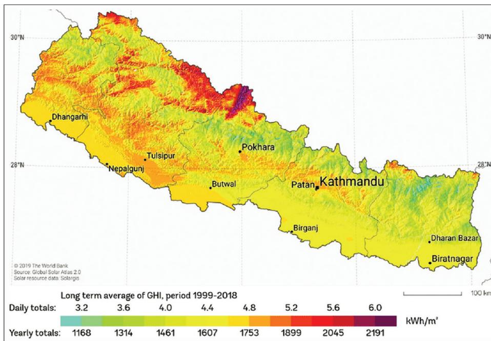
types of solar energy technology: grid-connected PV, solar water heaters, solar lanterns, and solar home systems. Nepal is located at a latitude of 26–30°N and experiences over 300 days of sunlight annually. The area has a rather high level of solar radiation, with an insolation of approximately 4.7 kWh/m<sup>2</sup> day (17 MJ/m<sup>2</sup> day). Additionally, it receives an average of 6.8 h of sunshine each day (SEMAN 2019).
